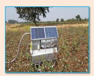
Solar base semi-automatic machine was developed by Ph.D student under guidance of NAHEP staff. This machine can pick 50 kg cotton in day. It is very cost effective and easy to use for farmers.
